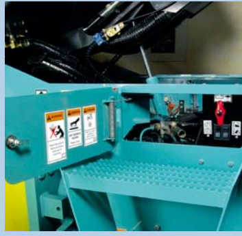
Tilting cabin for safe and easy maintenance and service
